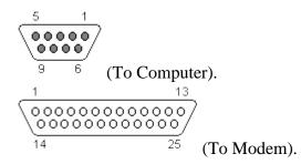
9 PIN D-SUB FEMALE to the Computer 25 PIN D-SUB MALE to the Modem
