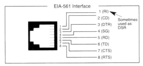
RS232D uses RJ45 type connectors (similar to telephone connectors)
