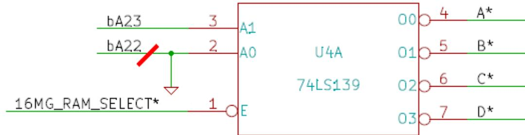
The diagram above shows the changes to U4A discussed above in schematic form, the red line indicates a cut in the signal trace bA22, pin 2 is then tied to GND.
