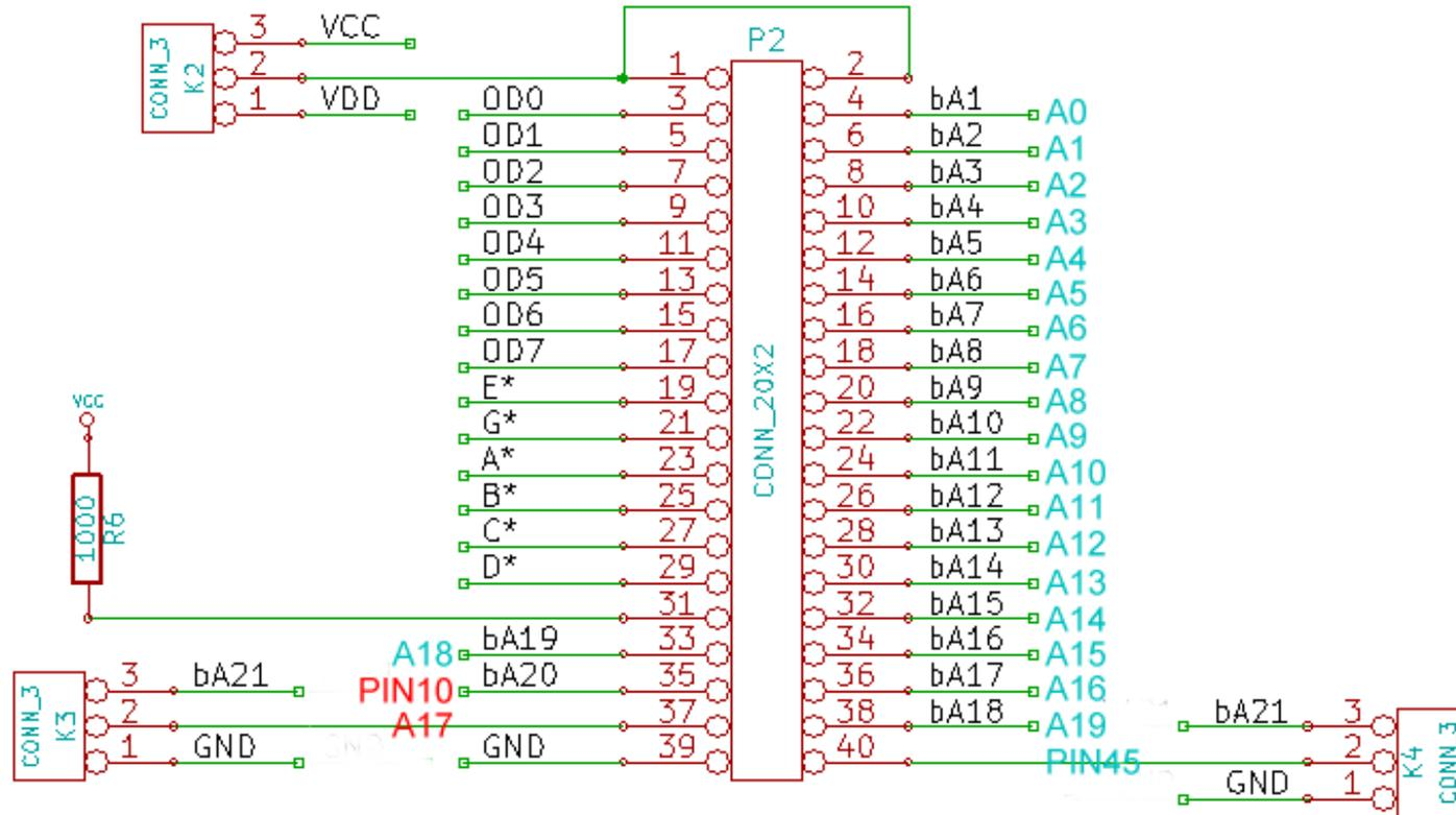
On the two diagrams above ignore the black 'net' names bA...etc, I have superimposed onto the connector pins the actual SRAM pinout to see how things line up with a V02 mezzanine (2<sup>nd</sup> March 2014) on the 16MB SRAM Board (23<sup>rd</sup> March 2014).
