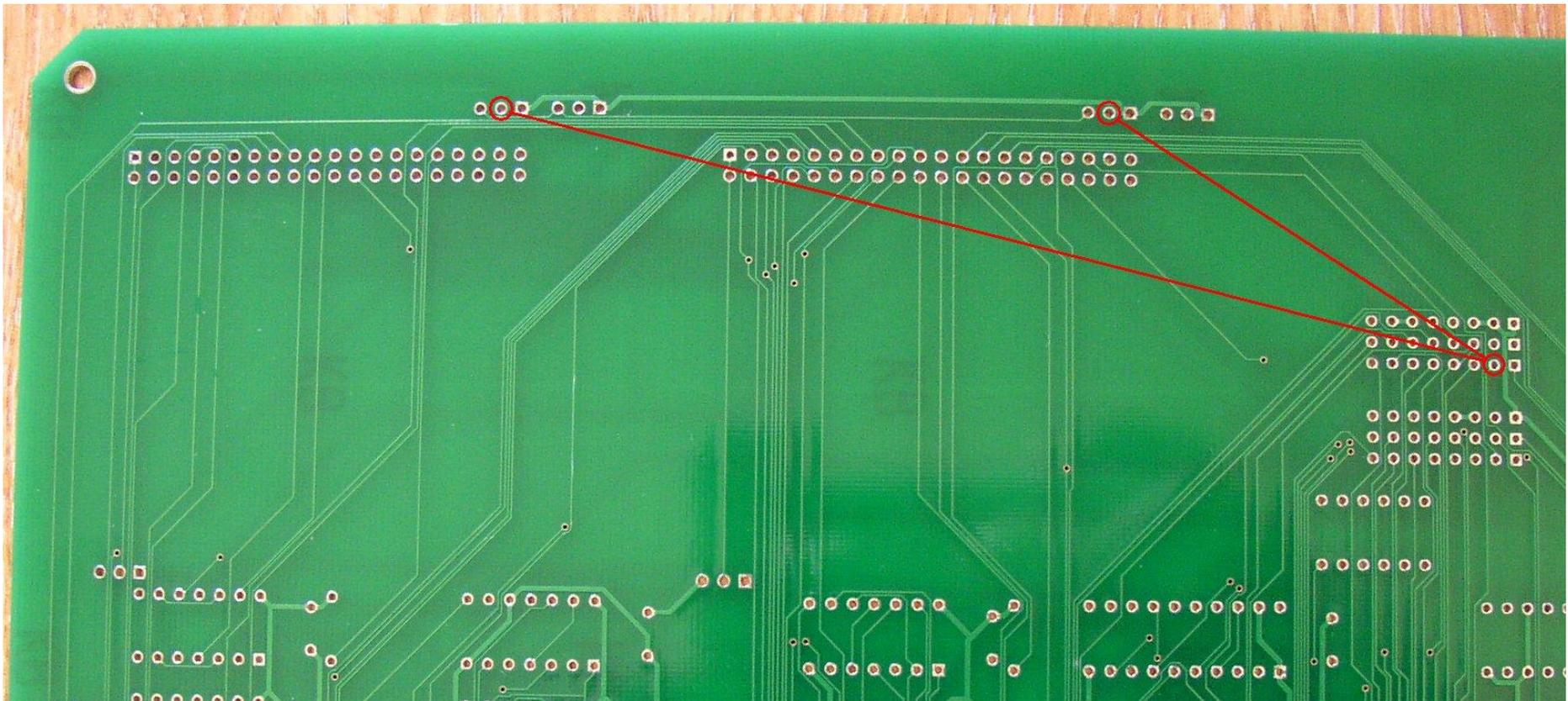
Finally solder 2 x AS6C3216 SRAM chips into locations U9 and U32 on each of the two mezzanines (4 chips in total) as shown in to picture below taking care to observe the correct orientation of Pin 1, mistakes are costly at \$22 approx per chip. Take care to ensure that the 16MB SRAM board is jumpered for 3.3v memory devices (K2, 1-2 and K5, 1-2) Then fit both mezzanines to the 16MB SRAM board and check other board configuration jumpers and set as necessary.
