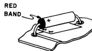
If the marking is the arrow type, orient the capacitor so that the arrow points to the negative polarity side. If the marking is one of the other two types, orient the capacitor so that the positive signs match the positive polarity side. Polarity is designated on the silk screened side of the board.
