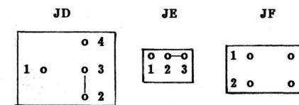
Shunt JD 2-3 Shunt JE 2-3 No shunts at JF Remove shunts A10 and A11 at JG
