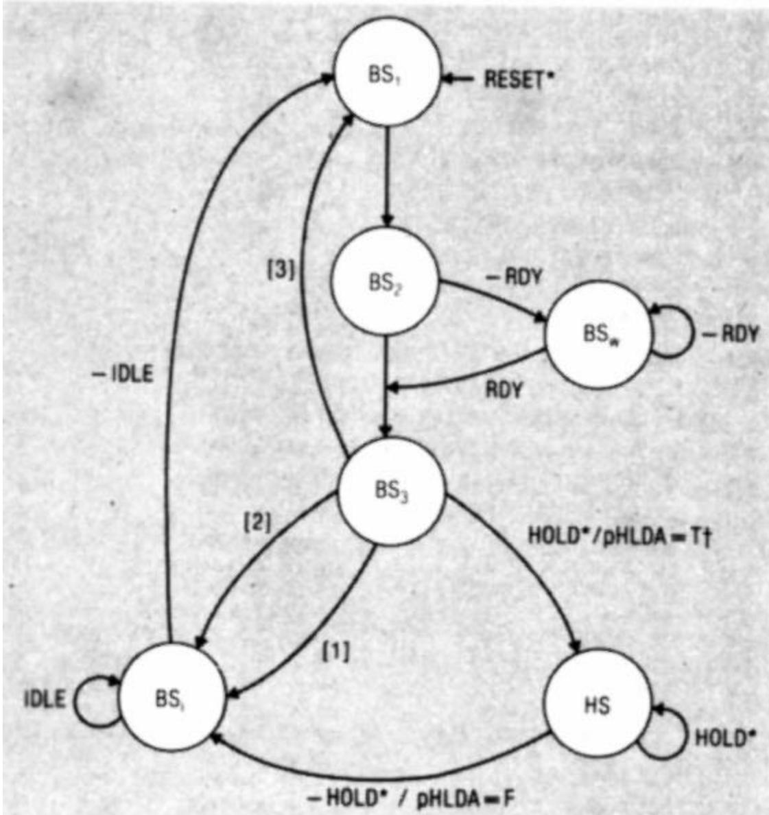
Figure 1. Permanent master state diagram.
