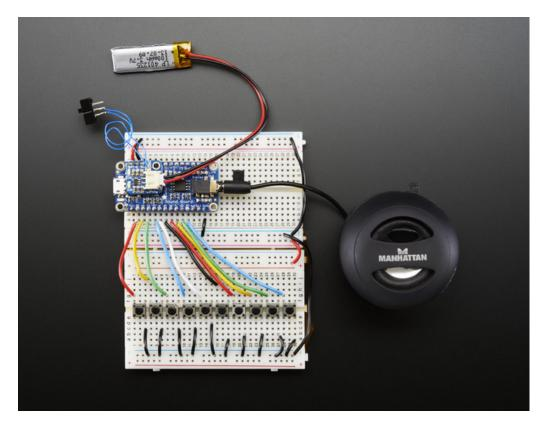
And a version with built in class D stereo amplifier, you can have 2 x 2.2W of output audio power, driving 4 or 8 ohm speakers
