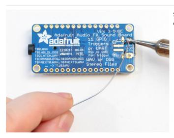
Start by melting some solder onto one of the side pads of the JST footprint on the bottom
