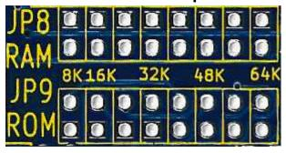
The onboard RAM can be selected in blocks of 8K by installing a jumper in that position. The onboard ROM is also selected in blocks of 8K, but since there is only 32K of ROM, it is duplicated for the upper half of the 8080's 64K address map.
