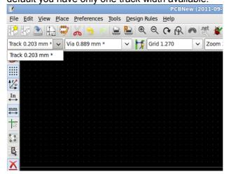
16. If you would like to add more track widths go to: Design Rules → Design Rules → Global Design Rules tab and at the bottom right of this window add any other width you would like to have available. You can then choose the widths of the track from the drop-down menu while you lay out your board. See the example below.
