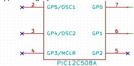
40. Some components have power pins that are invisible. You can make them visible by clicking on the 'Show hidden pins' icon on the left toolbar. Hidden power pins get automatically connected if VCC and GNS naming is respected. Generally speaking, you should try not to make hidden power pins.
