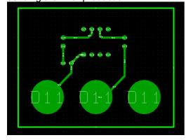
6. To generate the drill file, from PCBNew go again for the File → Plot option. Default settings should be fine.
