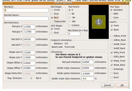
5. Set the 'Pad Num' to '1', 'Pad Shape' to 'Rect', 'Pad Type' to 'SMD', 'Shape Size X' to '0.4', and 'Shape Size Y' to '0.8'. Click OK. Click on 'Add Pads' again and place two more pads.
